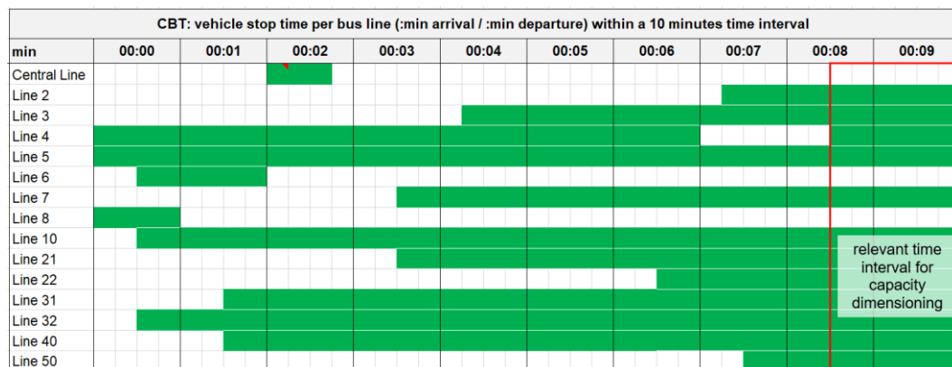
Figure 28: CBT: vehicle stop time per bus line (min of arrival/ min of departure) within a 10 minutes time interval
